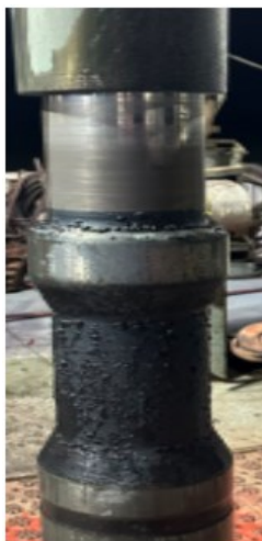
Figure 5: Sample Torsional Vibration Reduction Tool
